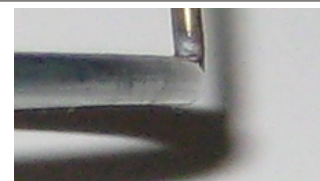
Clean, solid welds
